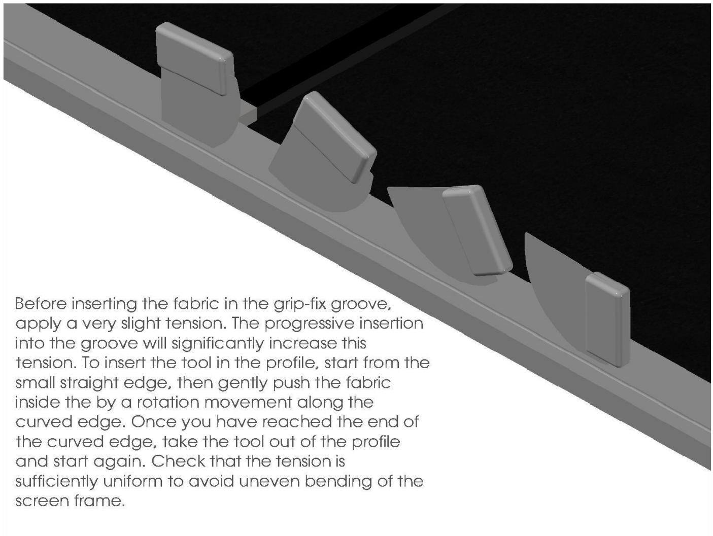
➤ Install the Enlightor fabric. Cut excess, leaving an edge margin of  $1/2"$ , fold fabric and using provided velvet finish sub frame edgings.
